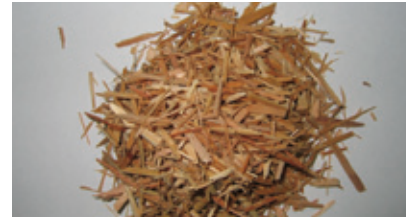
Wood chips (Construction scrap wood)
