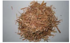
Wood chips (Construction scrap wood)
