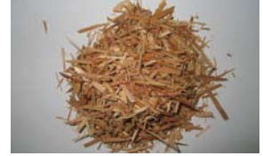
Wood chips (Construction scrap wood)
