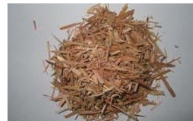
Wood chips (Construction scrap wood)
