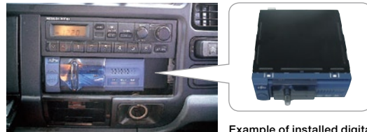
Example of installed digital tachograph
